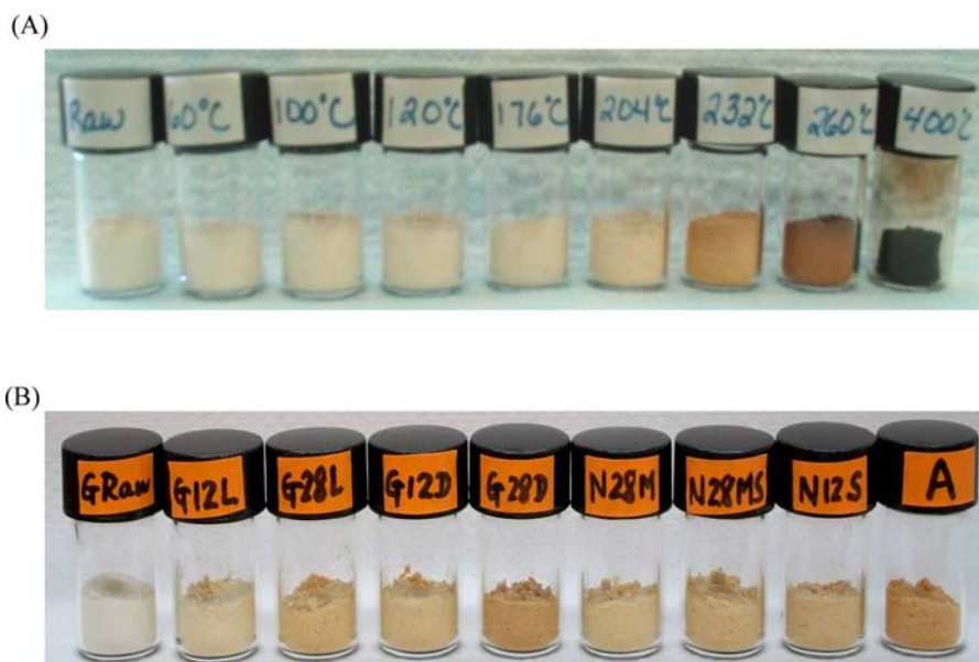
Figure 1. (A) Laboratory-prepared peanut flours subjected to dry-heat treatment for 10 min at different temperatures; (B) commercial peanut flour samples with different fat contents and different degrees of roasting. GRaw, Golden, raw; G12L, Golden 12% fat, light roast; G28L, Golden 28% fat, light roast; G12D, Golden 12% fat, dark roast; G28D, Golden 28% fat, dark roast; N28 M, Nutrin 28% fat, medium roast; N28MS, Nutrin 28% fat, medium-strong roast; N12S, Nutrin 12/14% fat, strong roast; A, company A.
